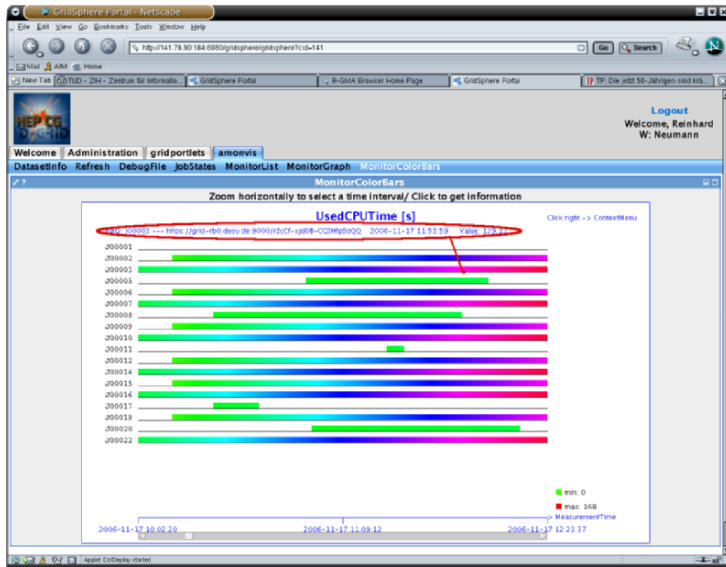
Figure 2. The monitoring is integrated into GridSphere. Here a example graph of the temporal development of an information (the CPU usage of the jobs). The red line and ellipse illustrate the interactivity - clicking in the display reveals more information. The ability to zoom in and out of the data is denoted by the scrollbars of the display.
